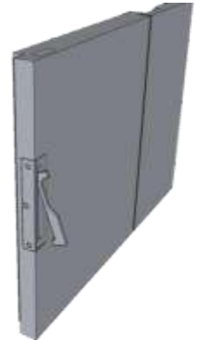
* Knife pull + Magnet catch (Outswing doors only)
